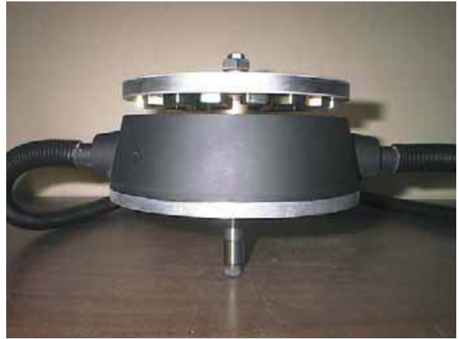
Like this Energy Systems & Design alternator from a Stream Engine turbine, many small, DC, hydroelectric units now use more efficient, brushless, permanent magnet alternators.
