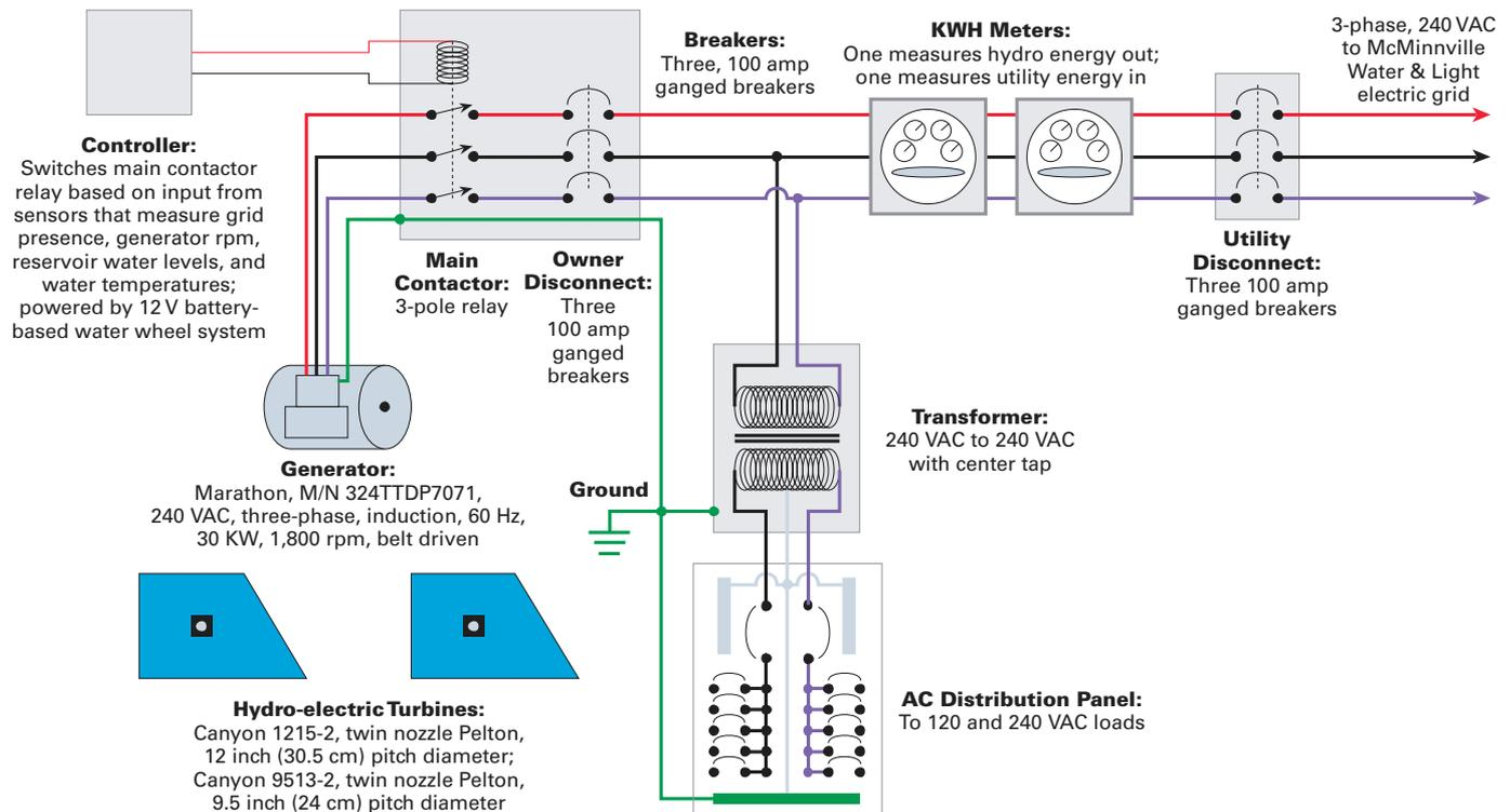
Since we have a net metering contract with McMinnville Water & Light, we cannot exceed 25 KW at any time during the year. Oregon law for net metering limits the output to 25 KW. This system is a three-phase, 240 V grid interface system that is wired directly into McMinnville Water & Light transmission lines. Electricity generated is credited by the utility through a net metering agreement signed earlier this year.
